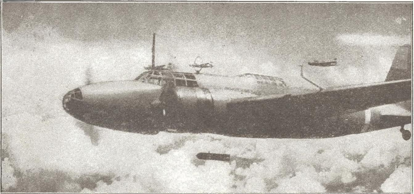
One of the latest and most modern of Japanese long-range bombardment types is the Nakajima 19. It uses two 870-h.p. Mitsubishi twin-row engines and has a top speed in excess of 250.
