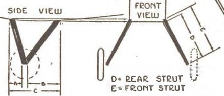
A THREE-VIEW DRAWING DOES NOT SHOW TRUE LENGTH OF THE VARIOUS STRUTS BUT THEY CAN BE DETERMINED QUITE EASILY AS ILLUSTRATED FOR A LANDING GEAR. USE SAME METHOD FOR WING STRUTS, ETC
