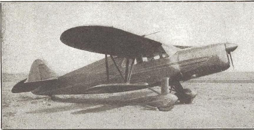
Menasco uses this Waco S Custom for testing engines. At the time of this test, the job was fitted with a C6-S4 of 260 h.p. Below: Our photographer was unable to learn the name of this new ship. The shot was snapped at Babylon, N. Y. If any readers have information on the plane we would like them to contact us.
