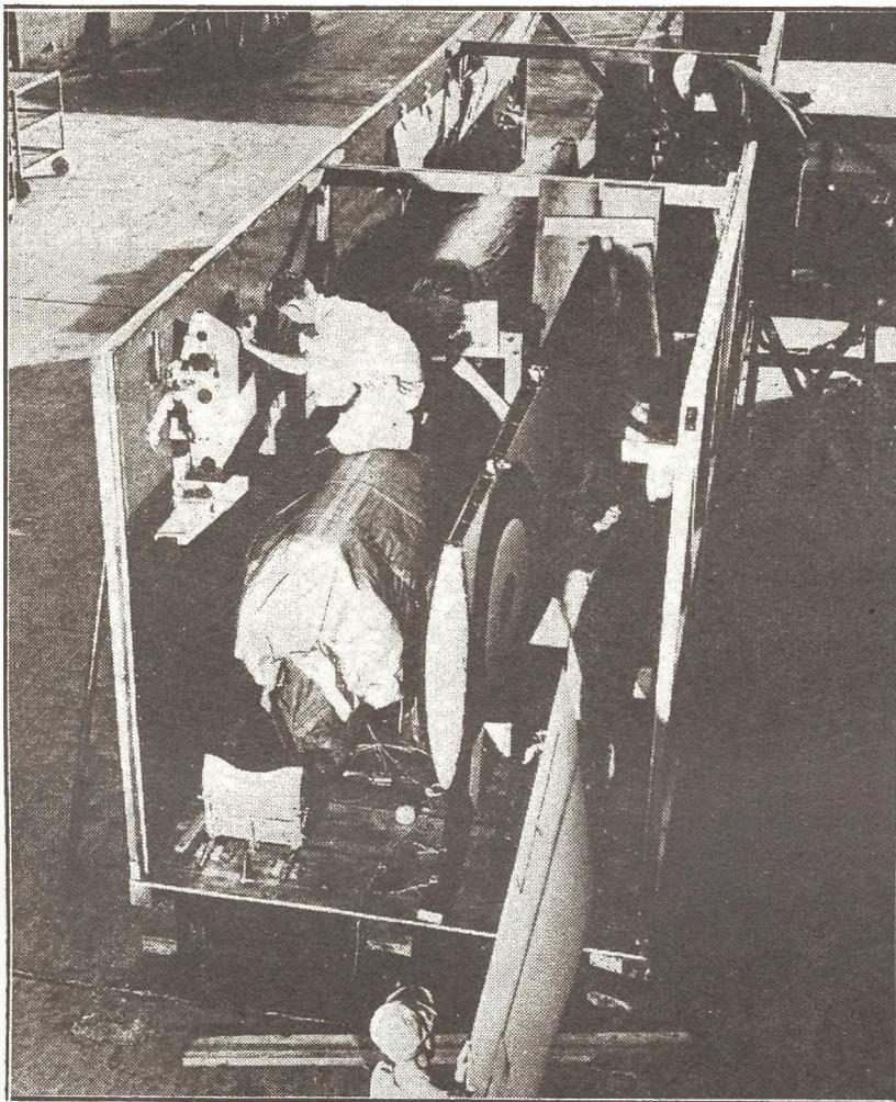
WORKMEN "wrap up" a very welcome Bundle for Britain—a Mustang fighter. This scene at the North American Aviation plant is typical of the efficiency with which planes of this type are crated for delivery by ship to the British. The Mustang's horizontal stabilizer is being pushed into its cradle in this picture. Note the slim fuselage, wrapped in heavy paper.
