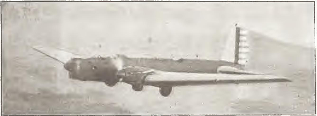
Here's a rare one for your scrapbooks. The Boeing B-9 heavy bomber was normally fitted with radial engines, but this one—the Y1B-9—used Curtiss Conqueror in-line plants. Note long, pencil-like fuselage and landing gear retraction system.
