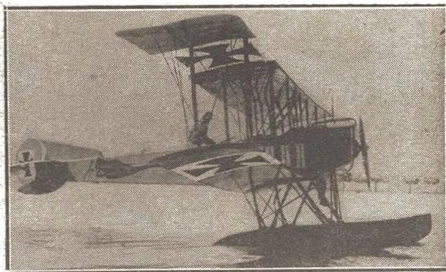
Seaplanes and flying boats of the Imperial German Navy carried pennant shaped streamers attached to the trailing edge of the lower wing. Note the streamer being blown back by wind.
